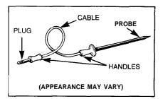
The temperature probe has a skewer-1'ike probe at one end and a plug at the other end that goes into a receptacle on the oven wall. Use handles of the probe and plug when inserting and removing from meat and wall receptacle. Do not use tongs to pull on the cable when removing the probe—they might damage it. TO AVOID BREAKING THE PROBE, MAKE SURE FOOD IS COMPLETELY DEFROSTED BEFORE INSERTING.
